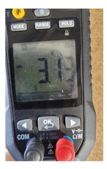
**1.Set Your Multimeter**: Switch your multimeter to measure **DC Volts**.
