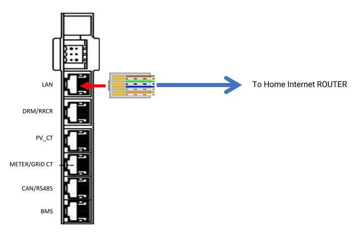
Next set a STATIC IP address for the ethernet connection
