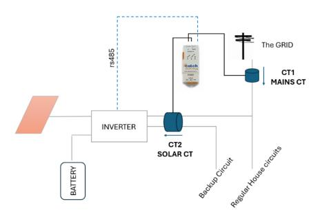
NOTE: How CT2 (W2) has the backup circuit and the AC Port of the inverter passing through it. If you cannot get both wires through one CT, you can parallel the two CT's into the W2 terminal, Just make the arrow on both CT's is pointing towards the inverter.
