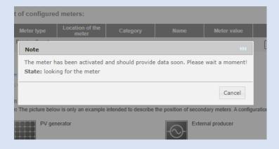
Once the inverter has successfully connected to the Solar Relay you will see this message.
